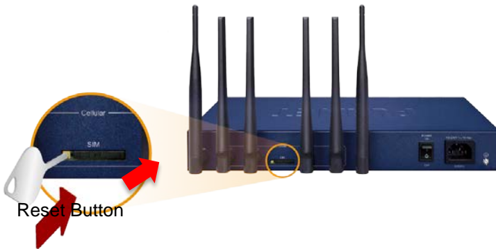
Figure 4-1: VR-300 Series Reset Button
