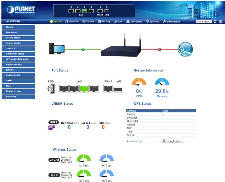
Figure 3-3: Web-based Main Screen of Cellular Gateway
